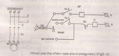
note : k: "start switch" RJ: heat relay C: AC contact
